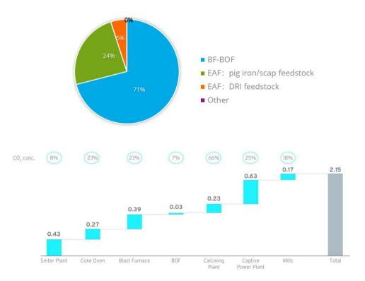
**70%** of the world steel production is based on Blast Furnace – Basic Oxygen Furnace (BF-BOF) route, that has a strong impact on the CO<sub>2</sub> production.
