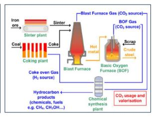
CDA includes technologies that avoid carbon emissions during steelmaking.
