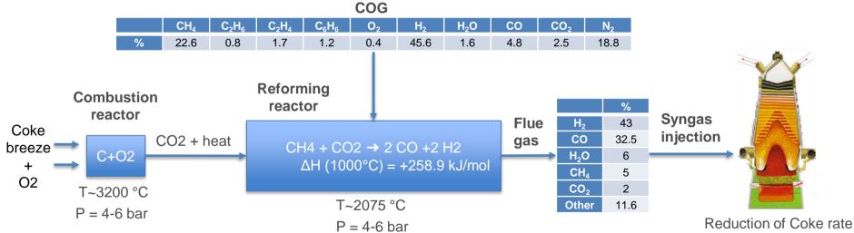
Main goal: H2-rich syngas with a H2/CO ratio (1.3 to 2) is 10 times higher than the hot decarbonated gas that is injected in the BF shaft in the TGR-BF process.
